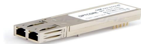
Fig. 6. External appearance of prototype with MPO receptacle.
