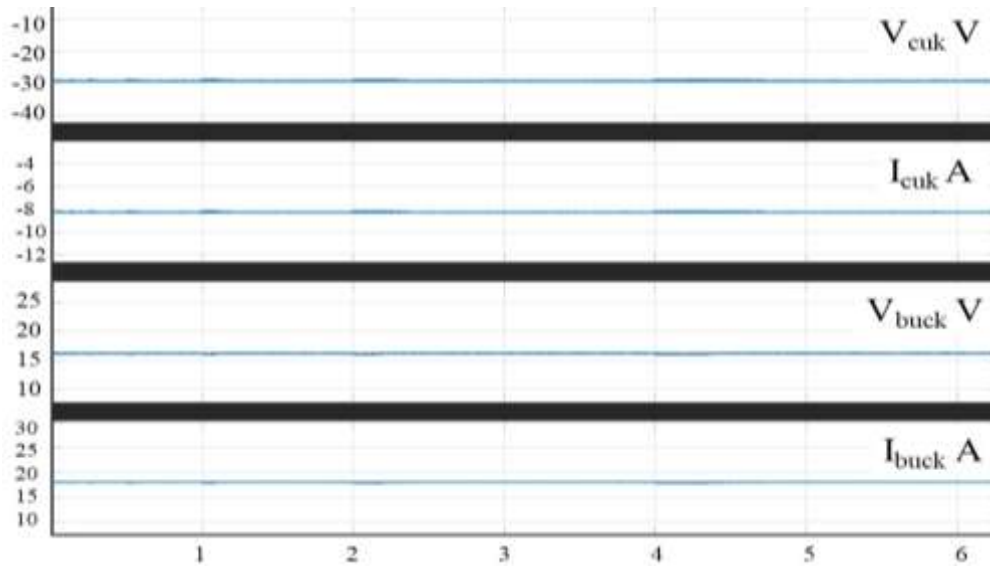
Figure 10. Output voltages ( V_{buck} , V_{cuk} ) and currents ( I_{buck} , I_{cuk} ) as a function of time for the tested Ćuk and Buck converters with PV input
